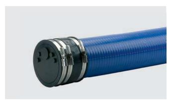
**KES-M 150-M-WE cable entry system**A seal at the empty conduit end can be created with a sleeve and a split interchangeable insert matching the cables that have already been laid. The sleeve is installed before the cables are laid. The entire cross-section of the cable entry system is available when laying the cables.
